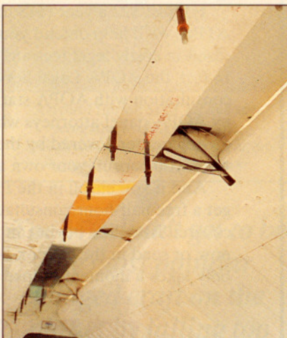
Stall fences (top) help lower stall speed. Optional flap seals (above) increase cruise speed. Aileron seals, already installed to the left of the hinge (below), improve roll control at low speed.
