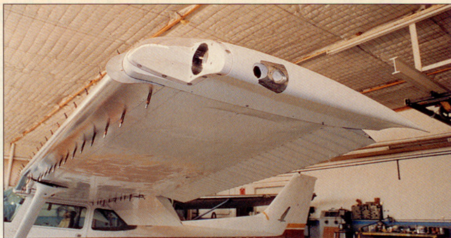
Horton's STOL kit can be made to accommodate the fiberglass RMD Aircraft wing tips. The wing tips accept the aircraft's existing strobes and navigation lights.
