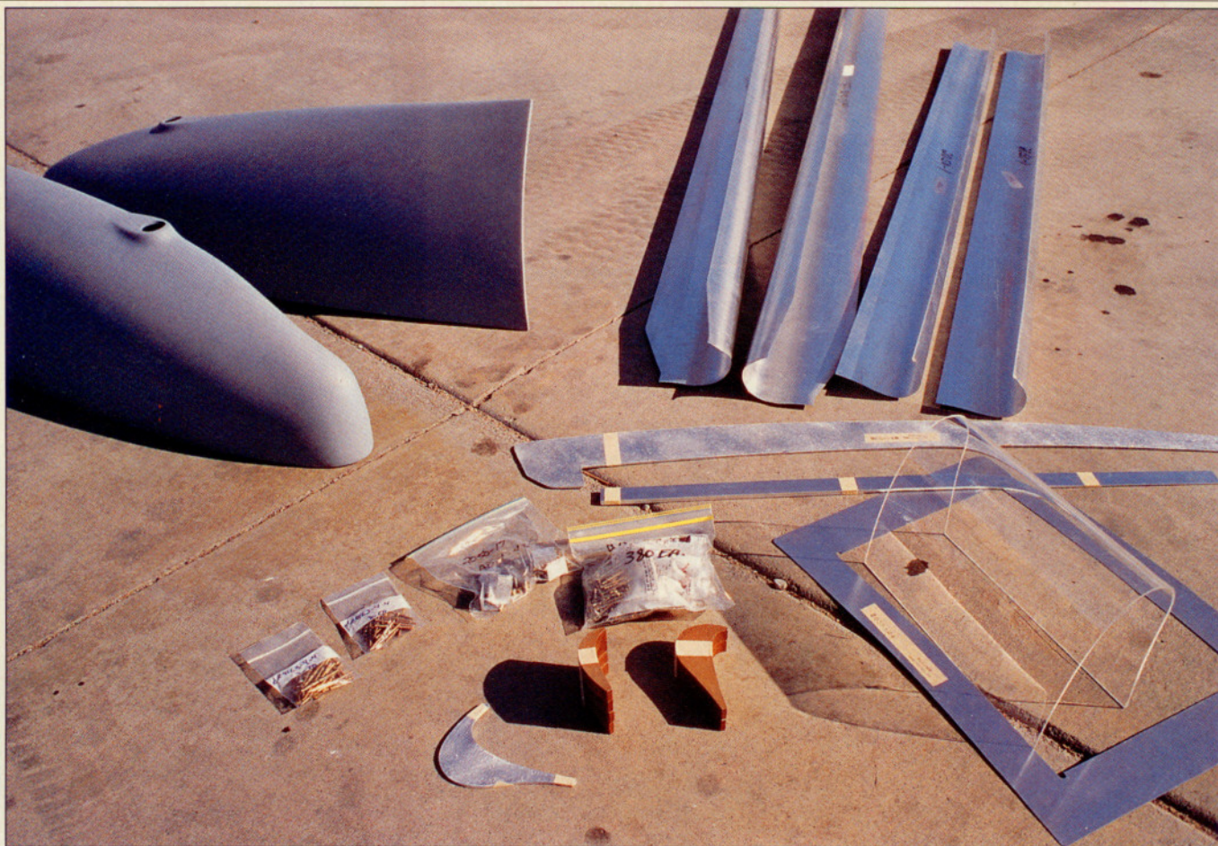
A typical Horton STOL kit includes wing tips, leading edge cuffs, stall fences, rivets, and, depending on the model, a landing light cover.
